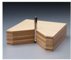
One of many proprietary Steinway & Sons innovations, the patented Octagrip™ pinblock can only be found in Boston pianos. The Octagrip™ pinblock is made of 11 layers of hard rock maple—glued in different grain angles of 60°—affording the tuning pins greater stability under tension and enabling the piano to stay in tune longer.
