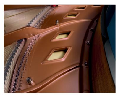
Every single piece of the piano vibrates while being played— except the plate, which is dedicated to a single function: ensuring total stability. Thanks to a special grey-iron material developed by Steinway & Sons— and its special vacuum fabrication—the plate can withstand the enormous string tension of several tons.
